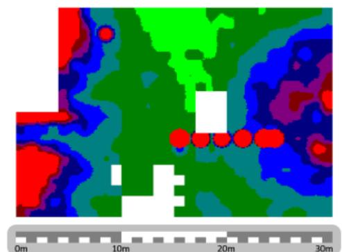
Figure 2: Resistivity plot showing five possible grave anomalies.
