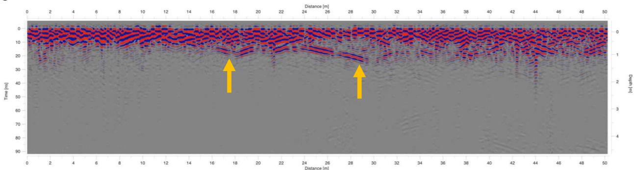
Figure 3: GPR Traverse showing possible sub-surface interface, possibly a grave.
