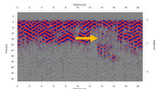
Figure 4: GPR profile showing evidence of buried wall foundations indicated by arrow.
