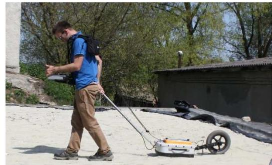
Figure 1: Charles Enright conducting a GPR survey. The GPR unit consists of an antenna that is pulled along the surface whilst continuously emitting a radar wave into the ground. When the wave comes into contact with a sub-surface interface part of its energy gets reflected to the surface. The time it takes for the wave to return can be used to calculate the depth of the feature/object.
